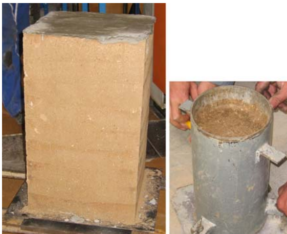
Fig. 5 Left: (40 \times 40 \times 65) cm 3 sample manufactured in the laboratory, surfaced on top with cement mortar. Right: cylindrical sample 16 cm in diameter \times 26.5 cm high
