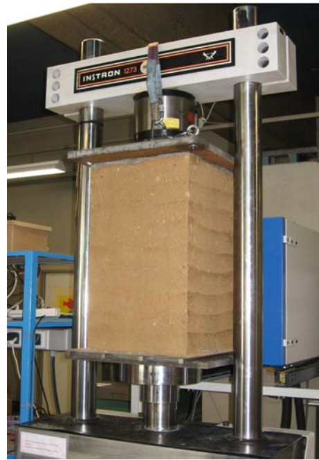
Fig. 6 Unconfined compression test of (40 \times 40 \times 65) \text{ cm}^3 sample
